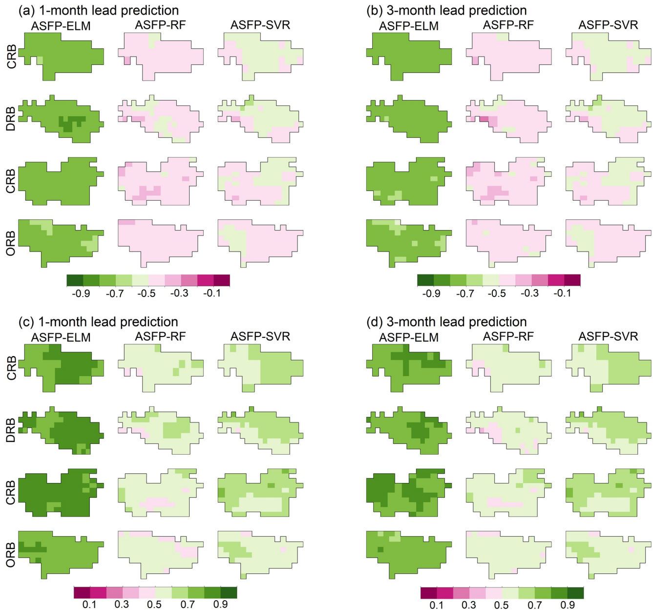
Figure 5. Correlation coefficients for probability (a and b) and deterministic (c and d) predictions of the three models in four river basins.
